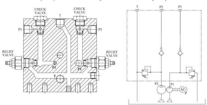
The W85AB series power pack is designed for applications that need two independent hydraulic power supply, but only use a single B14 Frame motor.
